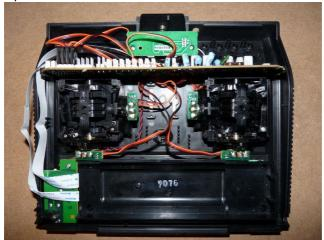
**2.** Mount the encoder with the 8 nuts tot he transmitter case.
